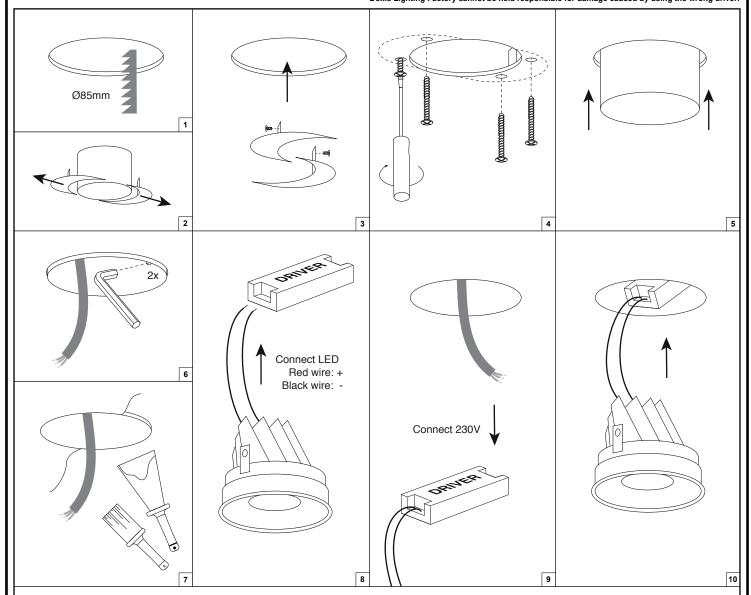
If cassette doesn't hold well inside trimless housing, clips can be bent outward a little bit.
